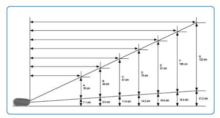
1. The screen height and diagonal length according to the projection distance
